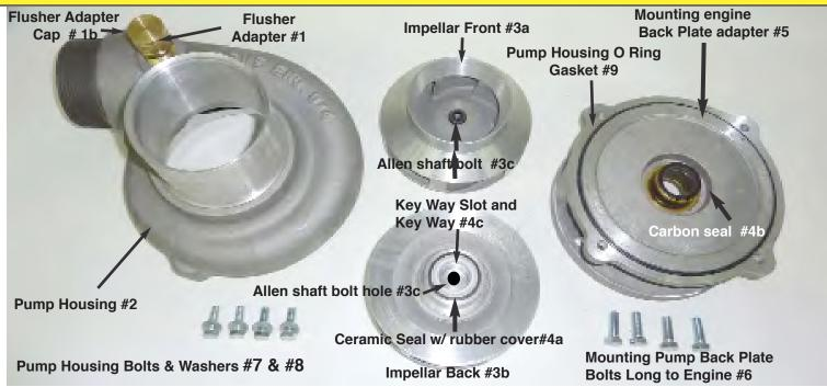
TOOLS REQUIRED: Standard Allen wrench 3/16ths. Standard 3/8 " & 1/2" open end wrench,
