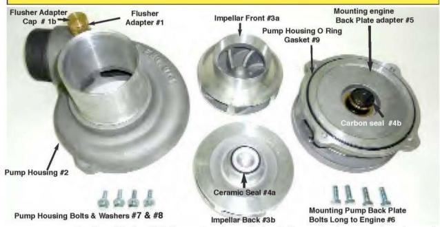
TOOLS REQUIRED: Small combination 1/2 inch wrench and a small tube of silicone adhesive to seat the carbon seal.
