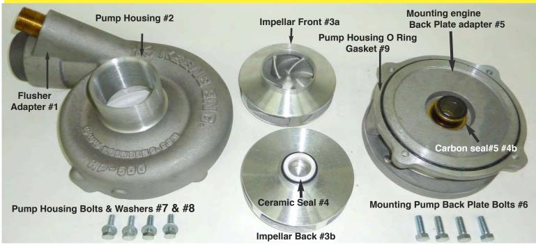
**TOOLS REQUIRED:** Small combination 5/16 inch and a 3/8 inch open end wrench.
