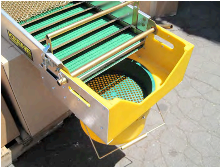
Assembled SBRS Bucket Mounted to Sluice Box
