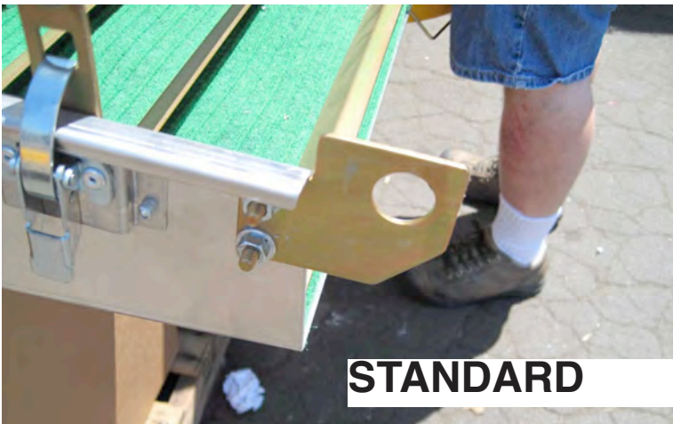
The SBRS Standard sluice mounting bracket mounts as shown. Align bracket at the top of the sluice fold and in against the sluice fold on each side. Clamp and drill two 5/16th holes and attach with bolts washer and nut.
